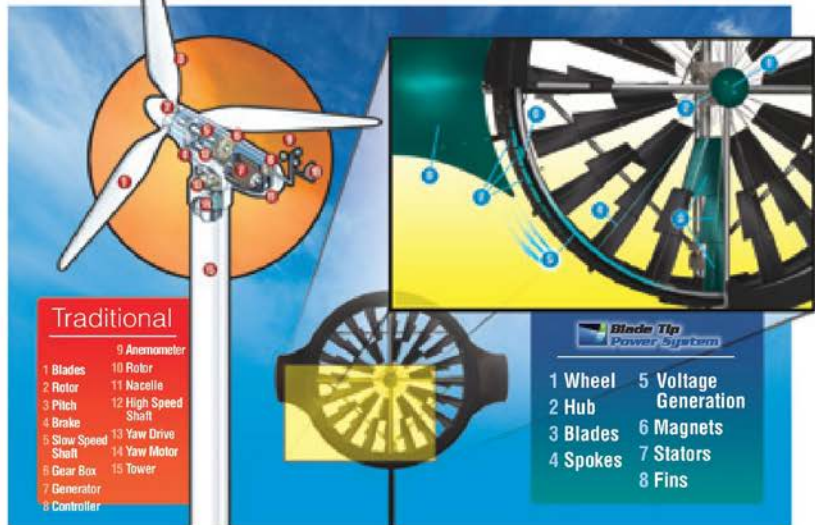
Turning a wind turbine into a wind generator by eliminating the gear box.
